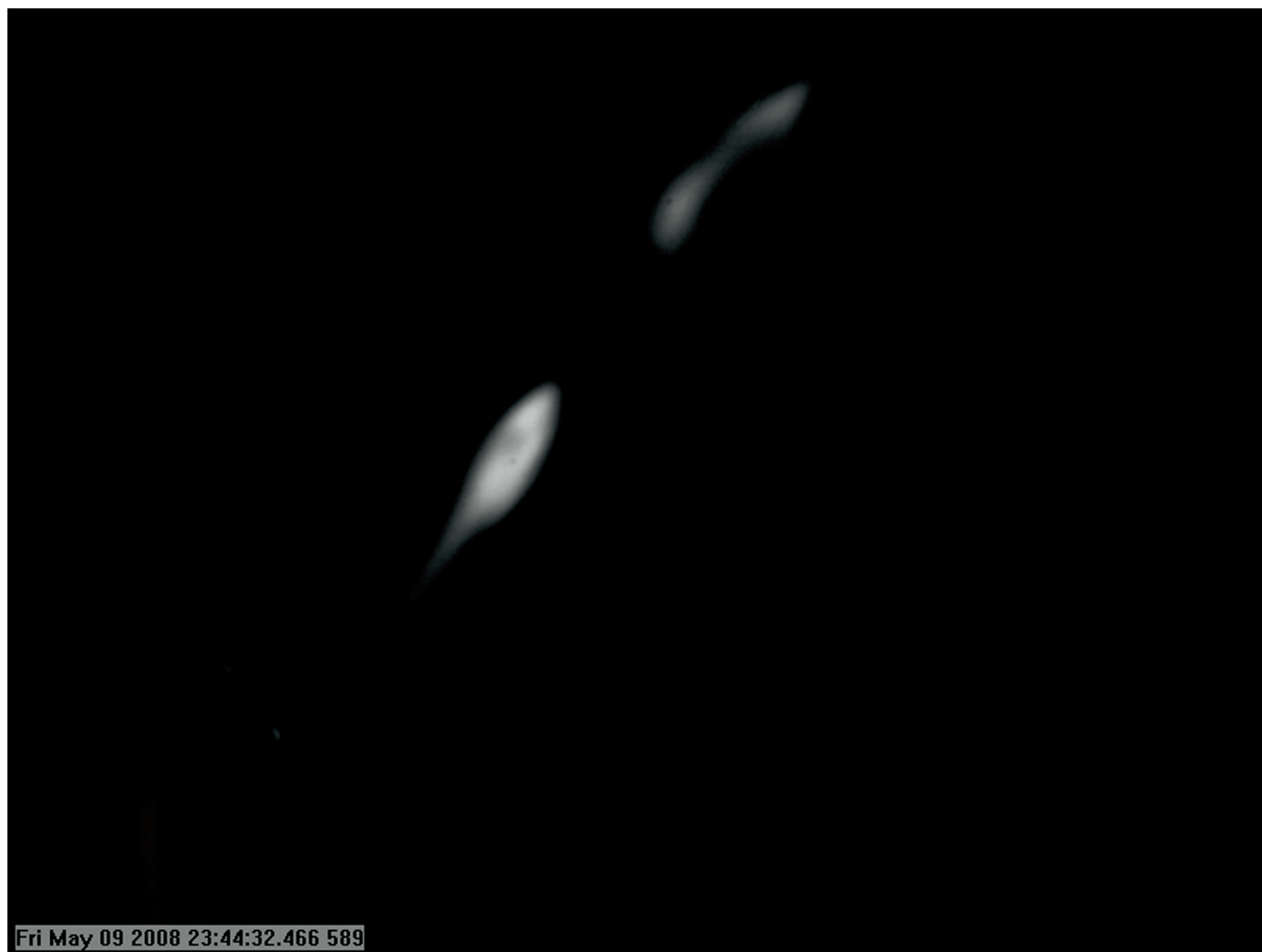
Movie S3. Recording 40-ms fluorescein pulses in substrate with plugs in chemistode. Fluorescence images were taken at 200 frames per second. The 9.1-s movie corresponds to 1.4 s of real-time imaging data.
